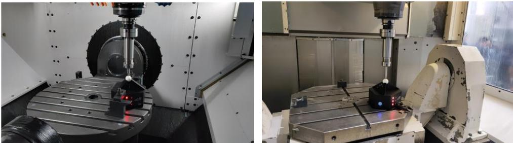
Fig. 15 On-machine measurement scene of prototype on MIKRON machine tools.
