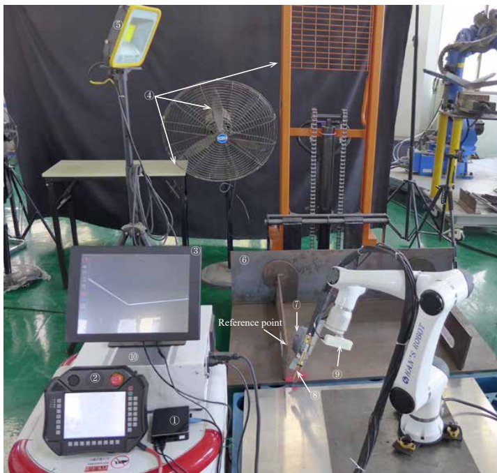
Fig. 16: Experimental workspace. ①Host computer ②Teaching pendant ③ Touch-screen computer ④Background interferers ⑤Fluorescent lamp ⑥Workpiece ⑦Laser-vision sensor ⑧Welding torch ⑨RGB-D camera ⑩Robot controller; (b) Outdoor experimental workspace.
