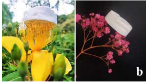
303 Fig.5. (a) Density and porosity of the SA/CMC aerogel and the superhydrophobic SA/CMC aerogel with 304 various concentration. Data are mean \pm SD (n = 3); (b) Optical images indicating the superhydrophobic 305 SA/CMC aerogel can stand on the top of flower stamens and dried flower.
