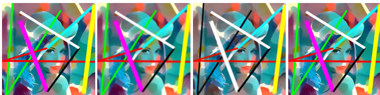
(b) Left to right: i. Stylized image with random Line Noise, ii. After applying Gaussian Filter, iii. After applying Median Filter, iv. After applying DnCNN
