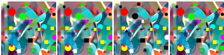
(c) Left to right i. Stylized image with random Shape Noise, ii. After applying Gaussian Filter, iii. After applying Median Filter, iv. After applying DnCNN
