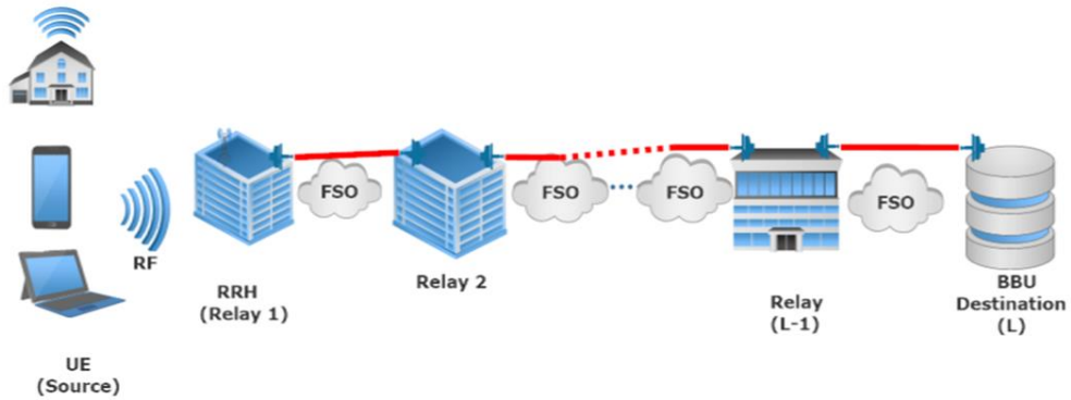
Fig. 1 Mixed RF and multihop FSO system with coherent detection
